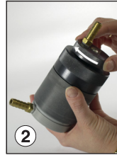
Thread calibration adapter into sampling head inlet.
