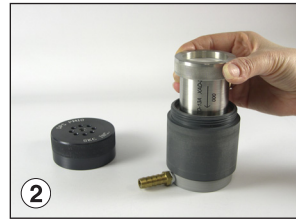
2 Lift media cartridge from cartridge holder section.
