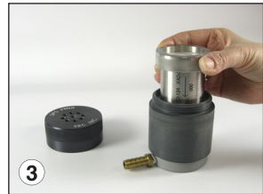
Insert media cartridge into cartridge holder section.
