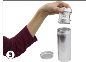
3 Wrap media cartridge in foil and insert in aluminum can.
