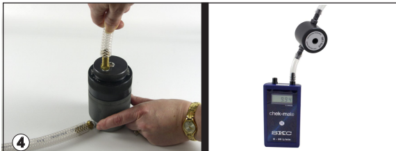
Use provided short length of calibration tubing to connect inlet of calibration adapter to outlet of a calibrator to form a calibration train. Note: SKC High Flow chek-mate Calibrator requires Pulsation Dampener Cat. No. 375-150 in line as shown at above right and in Step 5 (see Accessories).
